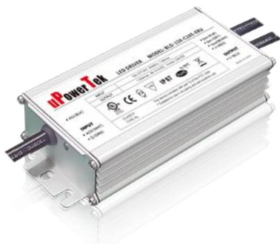
The global certified BLD-075-V series is a dual stage high efficiency smart LED driver. 2% minimum level and high frequency PWM output provides strobe flicker free user experience. 100khour long life and 7-year warranty provide high confidence to luminaire users. It supports not only traditional dimming control, but also DALI2.0 and other protocols. All around protections including digital OTP, SCP and OCP with auto-recovery secure 24hour non-stop operation for luminaires.
