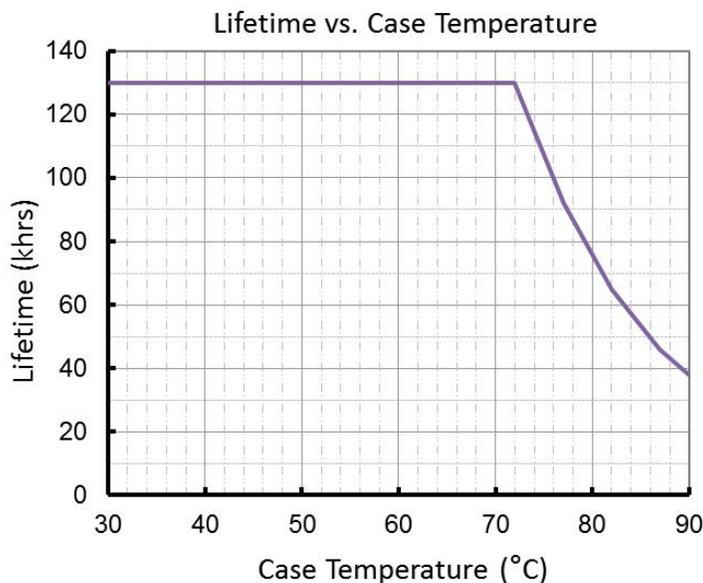
(End of Life: Maximum Failure Rate=10%)
