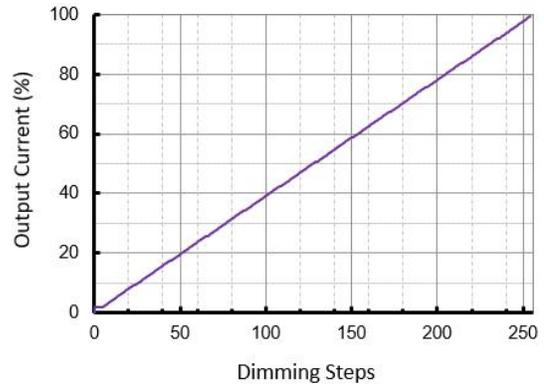
Note: Both DALI and DMX dimming curves can be customized to be linear or logarithmic as default.
